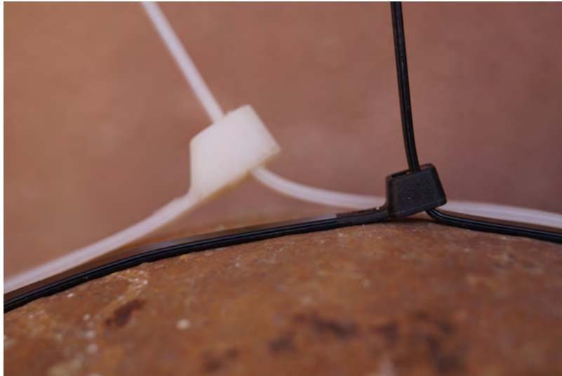
Figure 2. The space created when using one big zip tie (white) compared to when using many small ones (black). Photo by Helen M. Bardas
