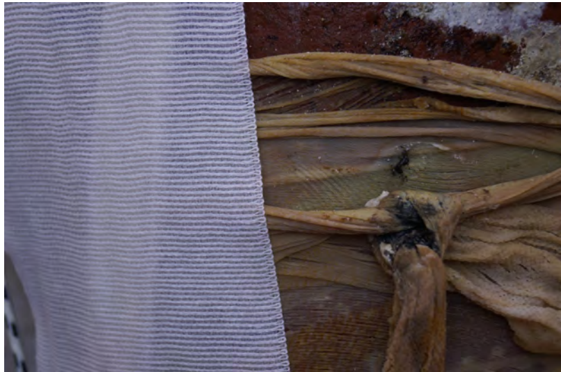
Figure 6. A fresh elastic bandage (left) compared to an elastic bandage after 8 months during the desalination process (right). Photo by Helen M. Bardas
